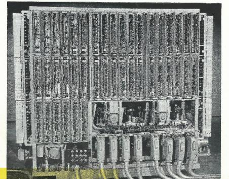
designated A, M, B, and Q. Adders are linked to registers A and Q. Registers M, B and Q are also used as immediate access stores. The four registers can transfer information to and from each other or the magnetic drum; shift numbers contained within registers; carry out testing functions on A, M and Q to allow the computer—depending on the conditions found—to branch along different paths of a program.
